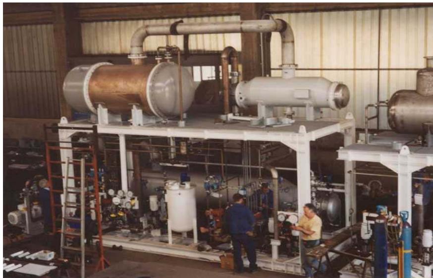
Package being shop tested
